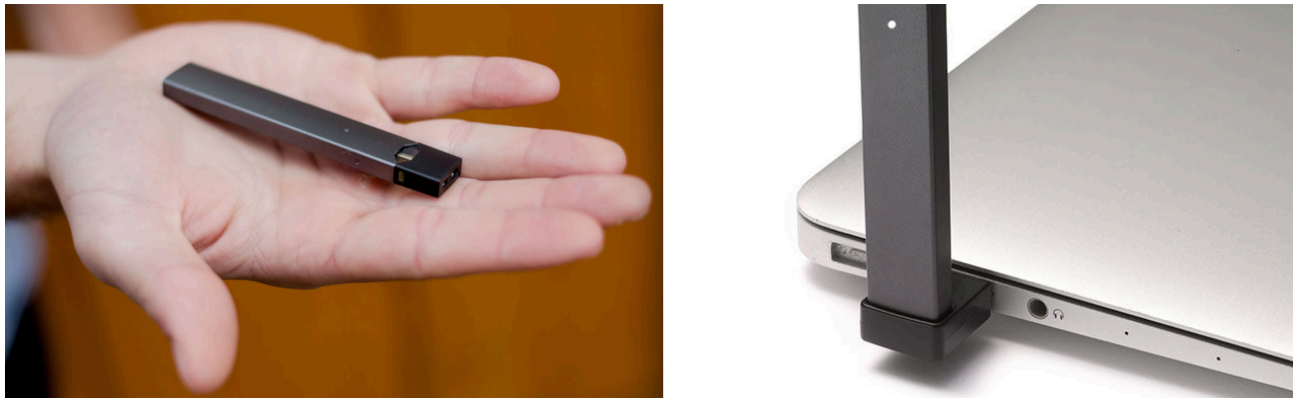
Figure 1: Left: Juul device as it fits in a palm (courtesy: UW Daily); right: Juul connected to a MacBook Air via a USB charger (courtesy: official Juul website)
