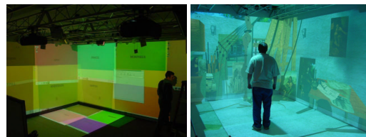
Figure 1. (a) arbitrarily placed overlapping projectors are (b) automatically calibrated and blended together so show a 3D model of Divinci's Workshop.
